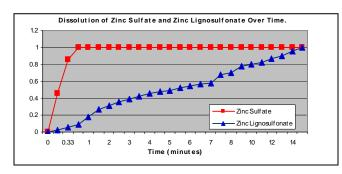
The amount of zinc applied was equal. Materials were applied to a slowly agitated solution (60 rpm) of de-ionized water. Dissolution was measured using electrical conductivity measurements of the solution
